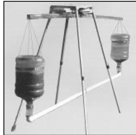
Figure 10. Liquefaction Demonstration. A ten-foot-long metal arm pivoted like a teeter-totter, with two 5-gallon bottles at each end, one filled with water, the other with various sediments, the two bottles connected by a pipe. Tipping the water end up forces water up through the sediments in the opposite bottle. Once liquefaction begins, plants and dead animals buried in the sediment container will float up through the sediments. Sedimentary particles fall or rise relative to each other and begin to sort themselves out into ever sharper layers of like particles.
